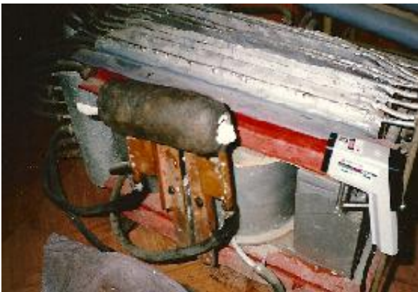
Fig.9. The inductor with the field concentrator in the heating process
