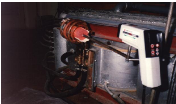
Fig.6. The double layer inductor in the heating process
